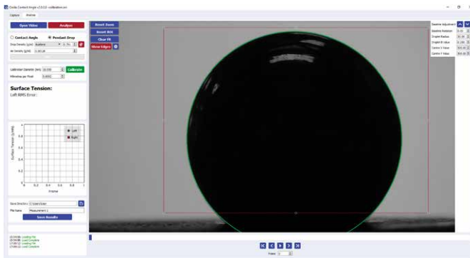
Figure 9.1. Calibrating the software using a calibration sphere.
