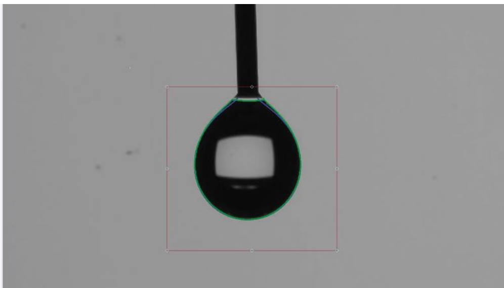
Figure 8.6. Surface tension measurement of a pendant droplet.
