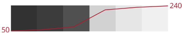
Figure 10.4. Lightness value change from 50 to 240, with a steep gradient between the central two pixels.
