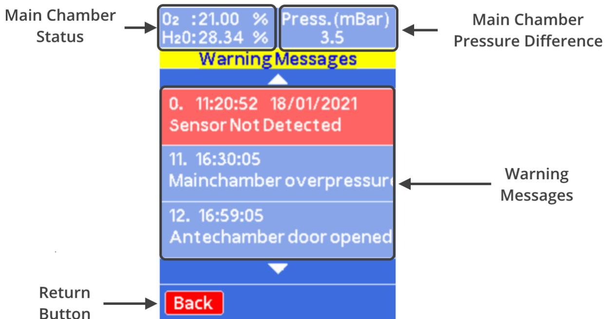
The warnings page has all the unread warnings that have occurred, these are time and date stamped so that the user can correlate it with working patterns within the glove box to help identify the reason for specific warning occurring. The warnings can be removed by navigating to a specific warning and pressing the OK button, this will delete them from memory. The warnings can be scrolled through using the up and down navigation arrows.
