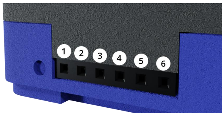
Figure 8.2. External interface header.
