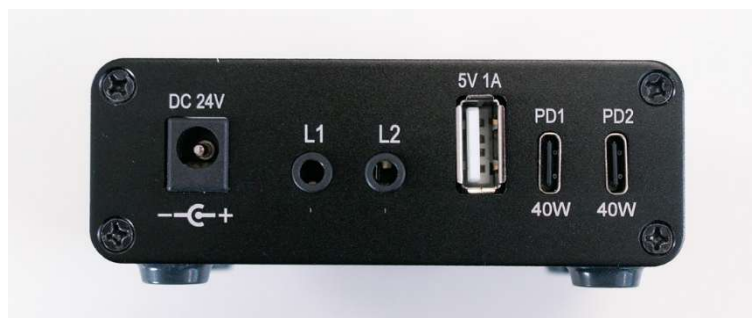
Figure 8.7. PSU rear panel showing the DC power input jack, two illuminator ports (L1, L2), a USB-A power port, and two USB-C power delivery ports (PD1, PD2).
