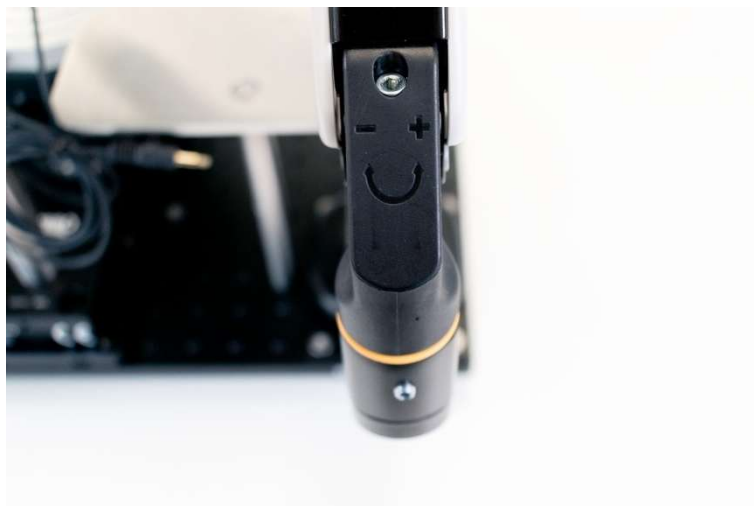
Figure 7.9. Monitor arm top piece installation and tension adjustment.
