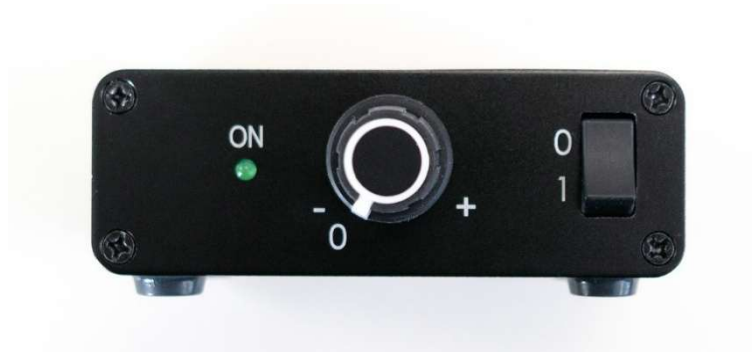
Figure 8.6. PSU front panel showing power indicator, illuminator adjustment knob, and power switch.
