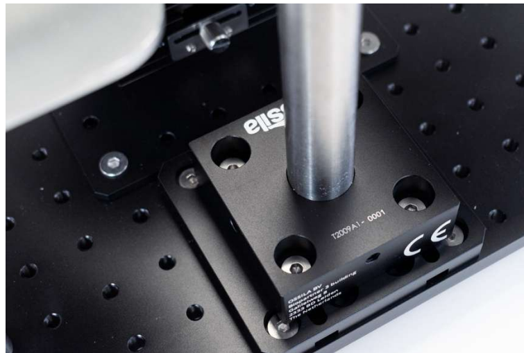
Figure 7.2. The microscope shaft mounting block, correctly installed on the base.
