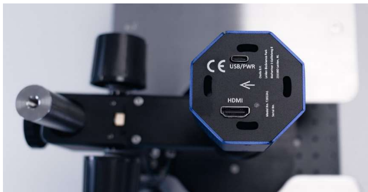
Figure 7.5. The microscope camera, correctly oriented to align the image and operator coordinates.
