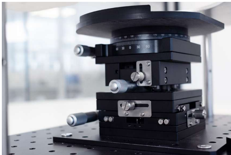
Figure 7.1. Probe Station translation stage, showing the X, Y, and Z stage lock screws.
