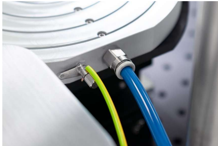
Figure 7.7. The vacuum chuck with 6 mm OD tube fitting on the vacuum line and a grounding wire for the chuck.
