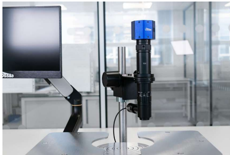
Figure 8.2. If the maximum stage travel is insufficient, the microscope can be swung left to right on the shaft to allow observation of the sample edges.
