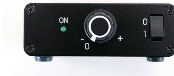
Figure 8.6. PSU front panel showing power indicator, illuminator adjustment knob, and power switch.
