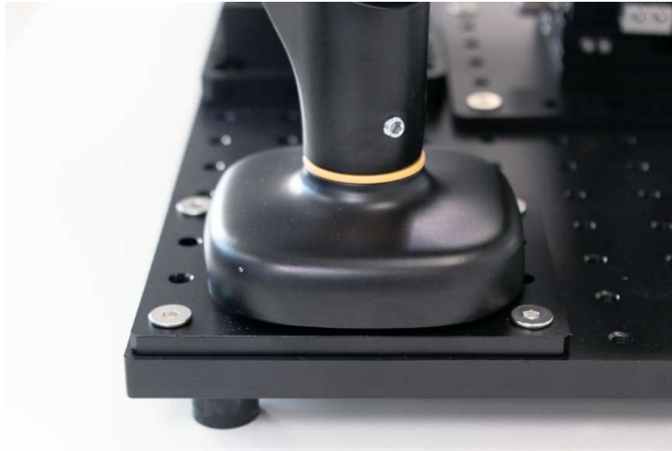
Figure 7.8. Monitor arm base plate mounting on breadboard.
