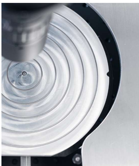
Figure 7.6. The vacuum chuck, correctly installed, with the tab of the chuck support aligned with the indent in the edge of the chuck.
