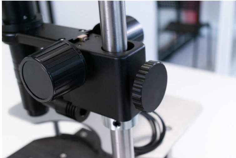
Figure 7.3. Microscope focus mount rear view, showing lock screw on the right, focus knob on the left, and the shaft collar underneath.
