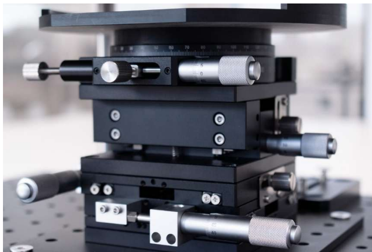
Figure 8.1. Details of the chuck translation stage, showing X, Y, Z, and R micrometer controls.
