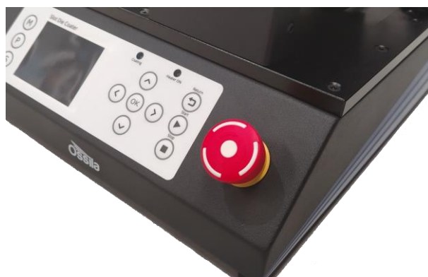
Figure 6.1 The emergency stop button mounted to the front of the slot-die coater.
