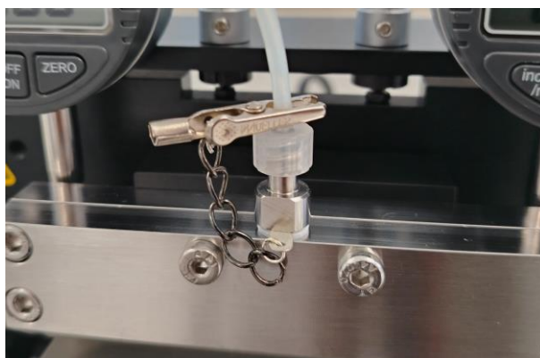
Figure 5.2 The slot-die coater tube clip and chain is used to secure the tubing
