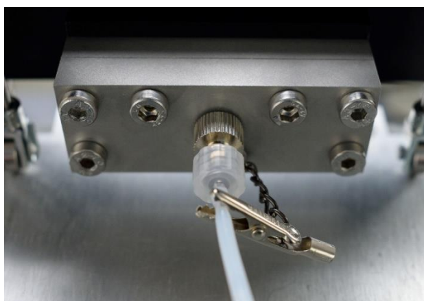
Figure 6.2 The slot-die coater tube clip and chain is used to secure the tubing
