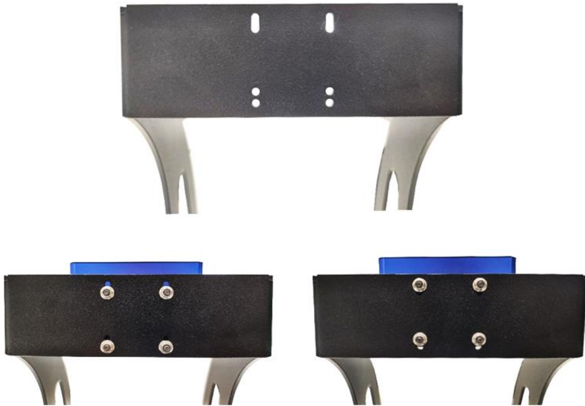
Figure 8.2. Bracket for mounting solar simulator on an Ossila Solar Cell I-V Test System - Automated. Left mounting is for 20 x 15 mm substrates, right for 25 x 25 mm substrates.
