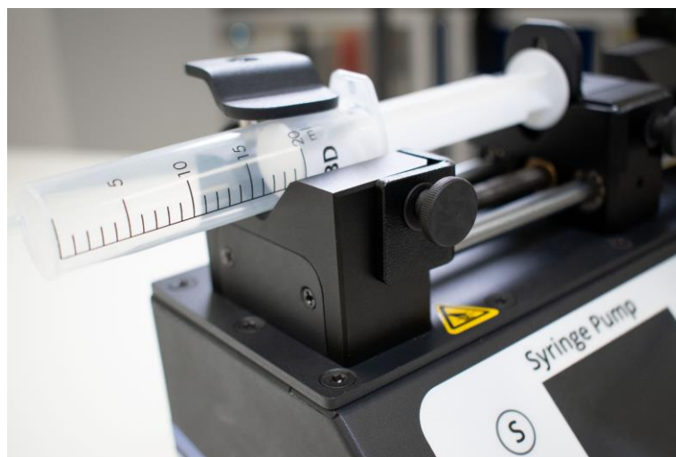
Figure 9.3. Placement of the top clamping arm
