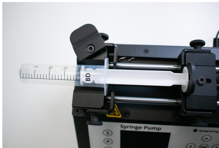
Figure 9.2. Placement of the syringe into the groove along with the barrel top placed in the clamping mechanism
