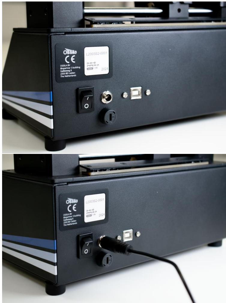
Figure 8.1 Installation of the Syringe Pump by plugging in the power supply cable.
