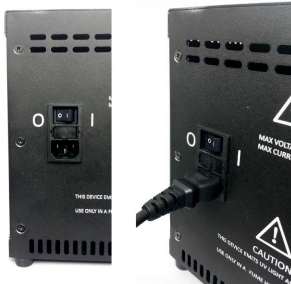
Figure 7.1. Installation of the UV Ozone Cleaner by plugging in the power cord cable.
